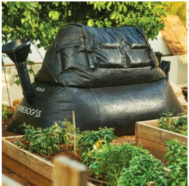
The HomeBiogas miniaturized anaerobic digester
