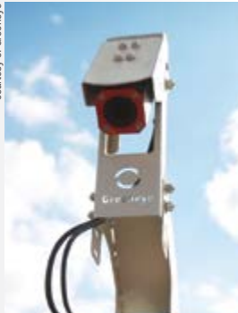
Greeneye images the field using cameras on the boom of a sprayer
