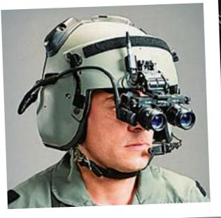
ANVIS HUD connects to the helmets of helicopter pilots, allowing pilots' heads to remain upright and looking out of the aircraft with all relevant information presented in front of the pilots' eyes.
