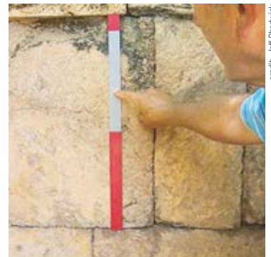
Measuring a stone ashlar block in an ancient wall with a special 54 cm “cubit” stick
