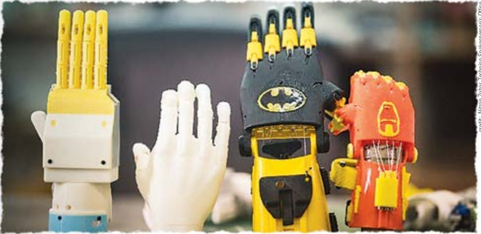
3D printed mechanical and robotic prosthetic hands
