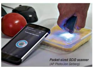
With the spectrometer, he said, you can just point the gadget at an item—without even knowing what it is. The device reads the item's molecular structure, matches the information to an ever-expanding database, and can send additional data to your smartphone.
